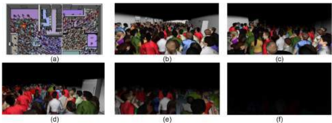
Fig. 14 Visibility of a person located at dance floor 1 (a) at 30 s (b); 60 s (c); 90 s (d); 105 s (e) and 135 s (f)
